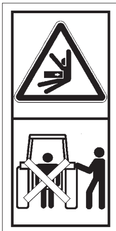
RISK OF CRUSHING
